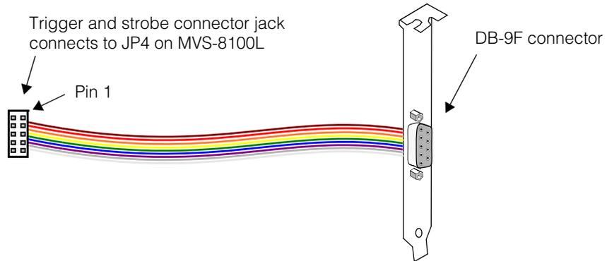
Figure 17. Trigger and strobe expansion panel P/N 800-0062
