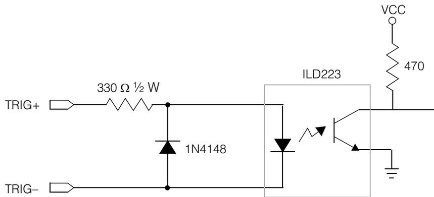
Figure 20. Trigger input schematic
