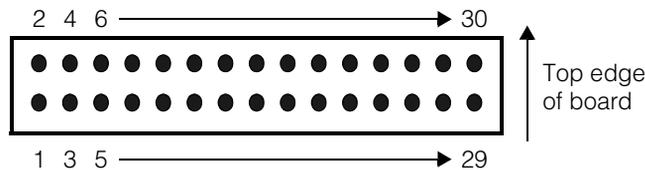
Figure 16. Pin numbering of camera expansion header, JP3
