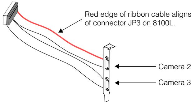
Figure 4. Location of pin 1 on camera port expansion panel
