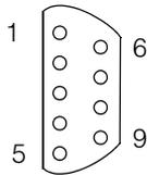
Figure 18. Pin numbering of the trigger and strobe DB-9F connector
