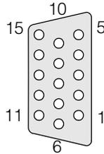
Figure 12. Pin numbering for camera port connectors
