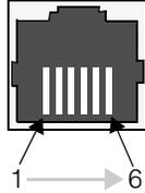
Figure 14. Pin numbering of RJ-12 jack for cable P/N 300-0178
